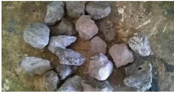
**Fig. 1: Ferrochrome Slag Aggregate**
